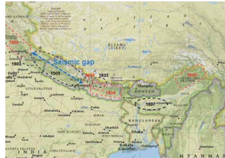
Rupture zones of major historical earthquakes in the Himalayan region and suspected "seismic gap" extending across west Nepal and eastern part of Uttarakhand state of India (base map prepared with NCEI/NGDC Natural Hazards Viewer)
